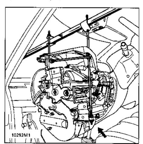
HERAUSZIEHEN DES ARMATURENBRETTES MIT DEM WERKZEUG Car. 1393.
