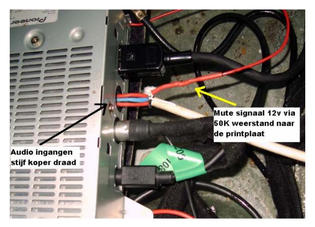
**Audio ingangen.....** = Audio input using stiff copper wire Mute signal via ..... = Mute signal to Radio MUTE via a 50K resistance soldered directly onto the circuit board.
